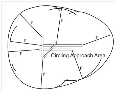
**Note:** Circling approach area radii vary according to approach category and MSL circling altitude due to TAS changes—see Figure 5-4-28.
